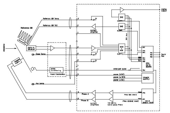
System Electronics Block Diagram
